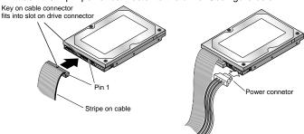
Note. If your computer does not have an unused power cable for your new hard drive, you can purchase a Y-shaped power splitting cable from your computer dealer which effectively converts one power connector into two.
