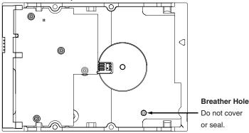
Caution. Do not cover, seal, or insert any object into this hole.
